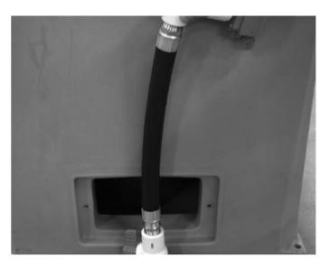
**Step 2**Attach the rubber hose and shutoff valve assembly to your incoming water line. Use teflon tape on all fittings to prevent leaks.
